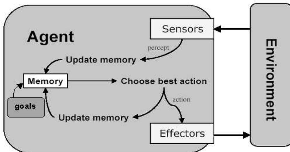
Figure 3-2. Interaction between agent and environment through sensors and effectors in the PAGE paradigm
