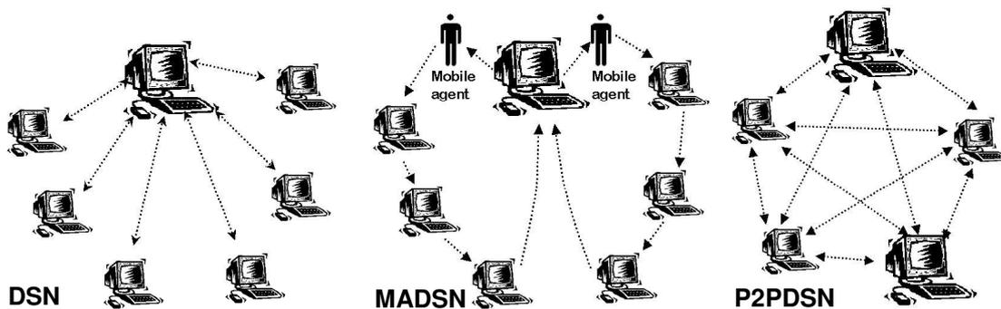
Figure 9-1. Architectures in DSN, MADSNS and P2PDSN
