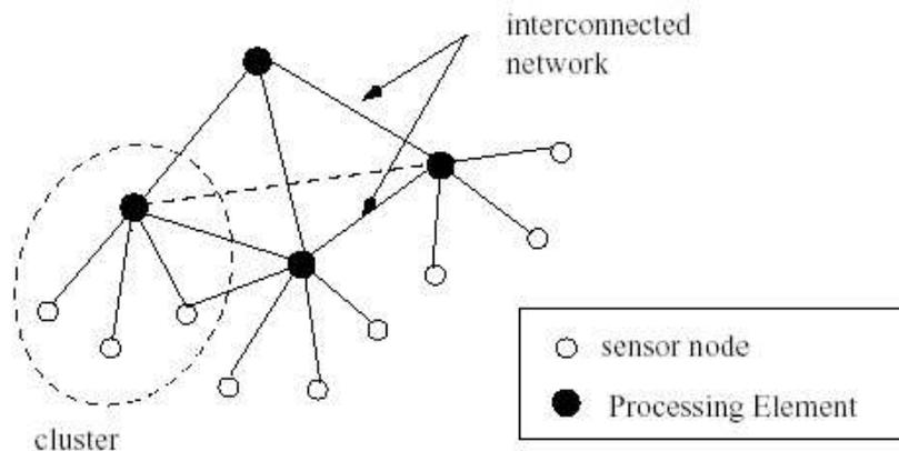
Figure 5-1 The architecture of a general DSN
