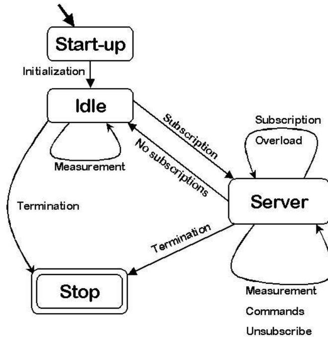
Figure 8-2. SA's state diagram
