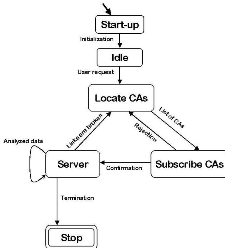
Figure 8-5. VA's state diagram
