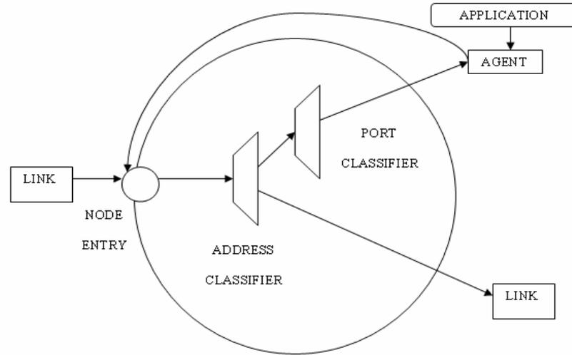
Figure 6.3 – Structure of node
