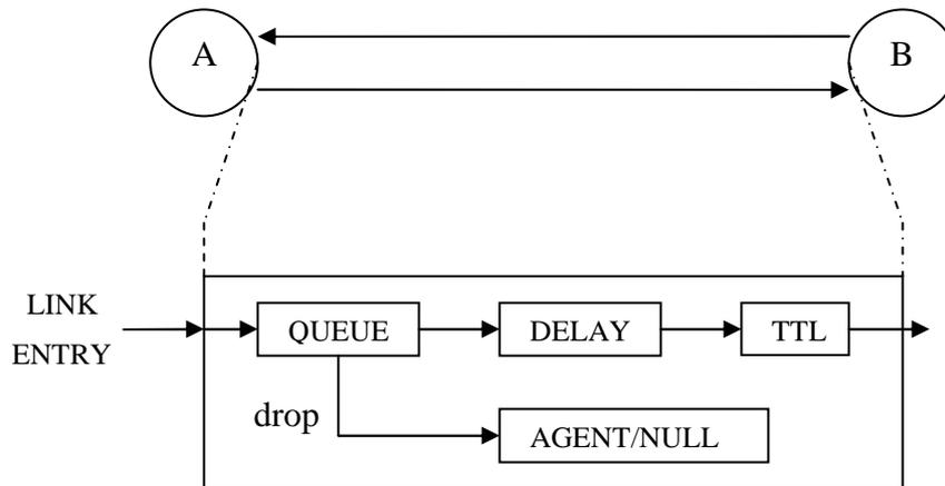
Figure 6.4 – Structure of link
