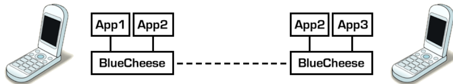
(b) BlueCheese makes a connection to another device with BlueCheese. Information about applications is exchanged and the applications that both devices have are informed (in this case App2) about the connection establishment.
